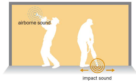
Figure 11.1 Airborne sound causes a structure to vibrate which causes it to emit sound on the other side.
