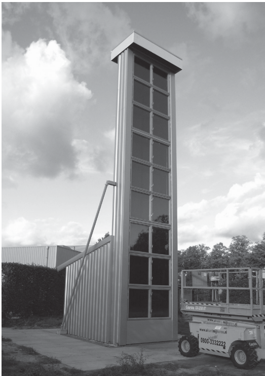
Figure 6.8 Experimental setup of a solar chimney (research by dr. B. Bronsema)
