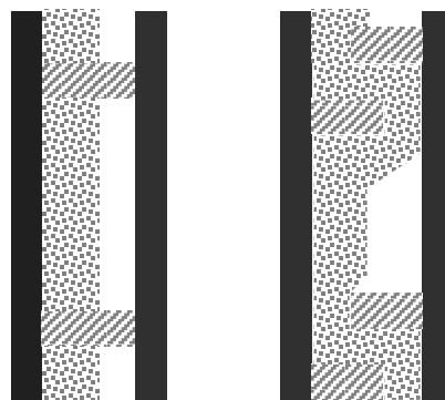
Figure 4.15 – Horizontal cross-section through a standard timber frame wall and a decoupled timber frame wall.
