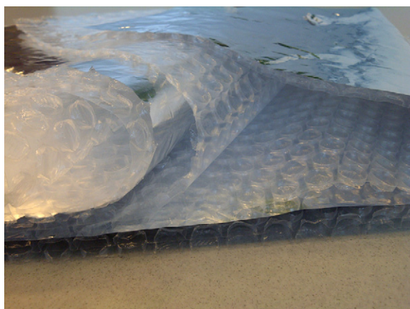
Fig. 1. Example of a reflective multi-foil insulation material.
