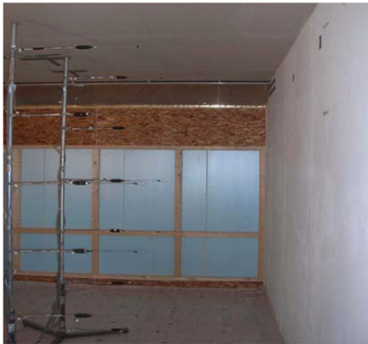
Figure 7: For a school this system has been adapted. Two air inlets are placed above each other (the silverish horizontal lines high in the back wall) and a spoiler has been added to it (shown in drawing). The air is preheated till 0 °C or more by two pipes. This system will be combined with thermally activated concrete floor above. The picture is from a test chamber in a laboratory of Cauberg-Huijgen Consulting Engineers, Zwolle. To prevent frost of the pipes in case of system failures, a water-glycol mixture is used as a heating medium. The system was applied in the ROC of Twente. During the night, etcetera, the inlet is closed off automatically in order to save energy and to improve temperature control.
