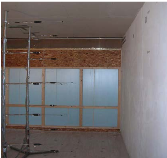
Figure 5: For a school this system has been adapted. Two air inlets are placed above each other (the silverish horizontal lines high in the back wall) and a spoiler has been added to it (not shown in the picture, see drawing). The air is preheated till 0°C by two pipes. This system will be combined with concrete core activation. The picture is from a test chamber in a laboratory of Cauberg-Huijgen Consulting Engineers, Zwolle. In order to prevent frost problems of the pipes in case of system failures, a water-glycol mixture is advised.
