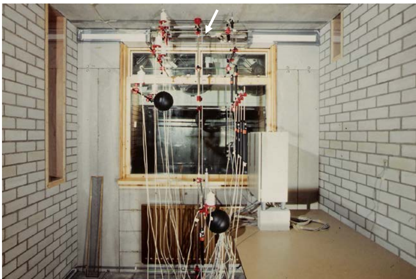
Figure 4: Option of air supply without draught ( DR < 20\% ) with an air inlet just beneath the ceiling (in the picture the white arrow in the back of the room). With an air inlet element length = 1 m, height = 20 mm > 45 l/s, 0^\circ\text{C} per m can be supplied. In order to have a low air resistance it is recommended to make use of a venturi shape of the air inlet. The picture is from a test chamber at the Delft University of Technology (4), with measurement equipment for velocity and turbulence, temperature, etc. The air supply makes use of the venturi principle (shown at the right of the picture, not shown in the picture itself).
