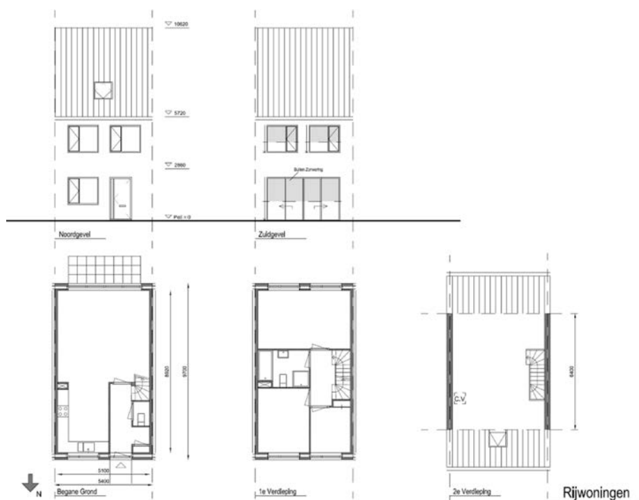
figure 4-1: Façade and floor plans of the reference dwelling (Single family terraced house)
