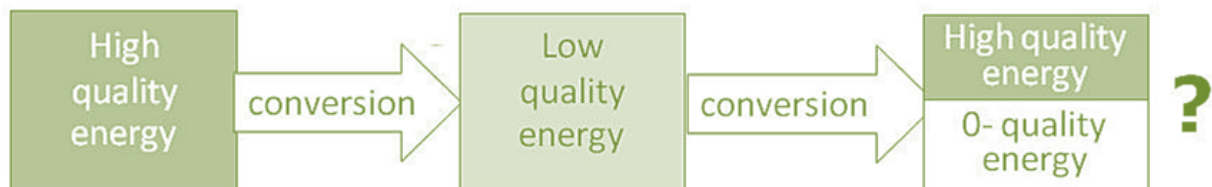
Figure 2-7: Not ideal conversion of high-quality energy into low-quality energy and vice versa.
